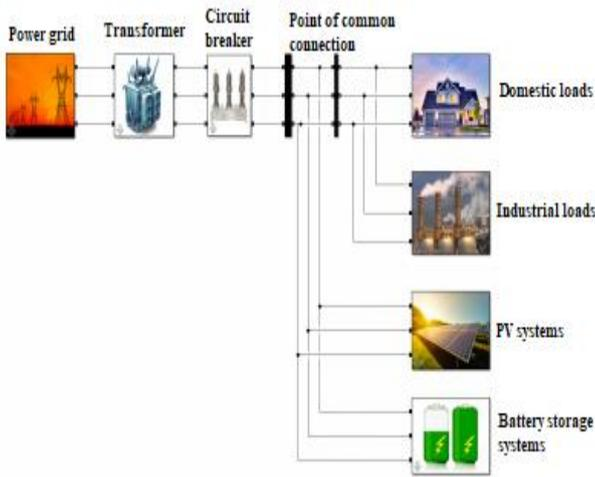
Fig. 2: Block diagram of the HMGS
