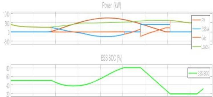
Fig. 4. Simulation result for a clear day using heuristic method
