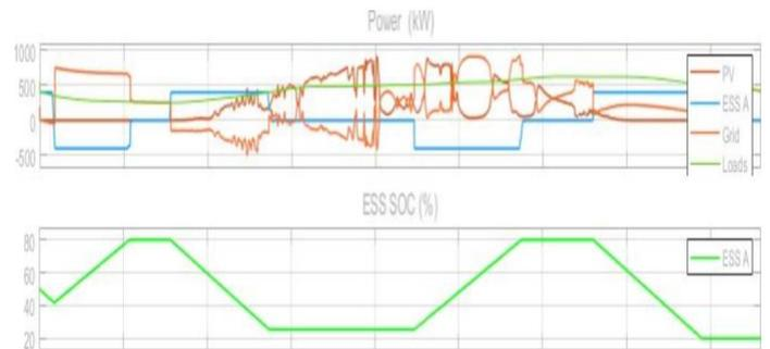
**Fig. 7:** Simulation result for a cloudy day using optimization approach
