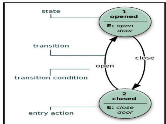
Fig. 3: Example of machine state logic for a door
