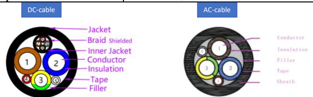
Fig. 9. DC/AC-Charging cable [32].
